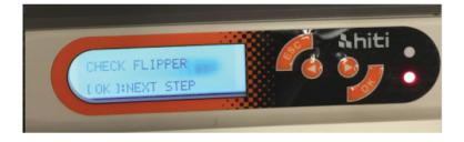
Step 3: Check if there is a card jam at flipper and click "OK" to remove it.
